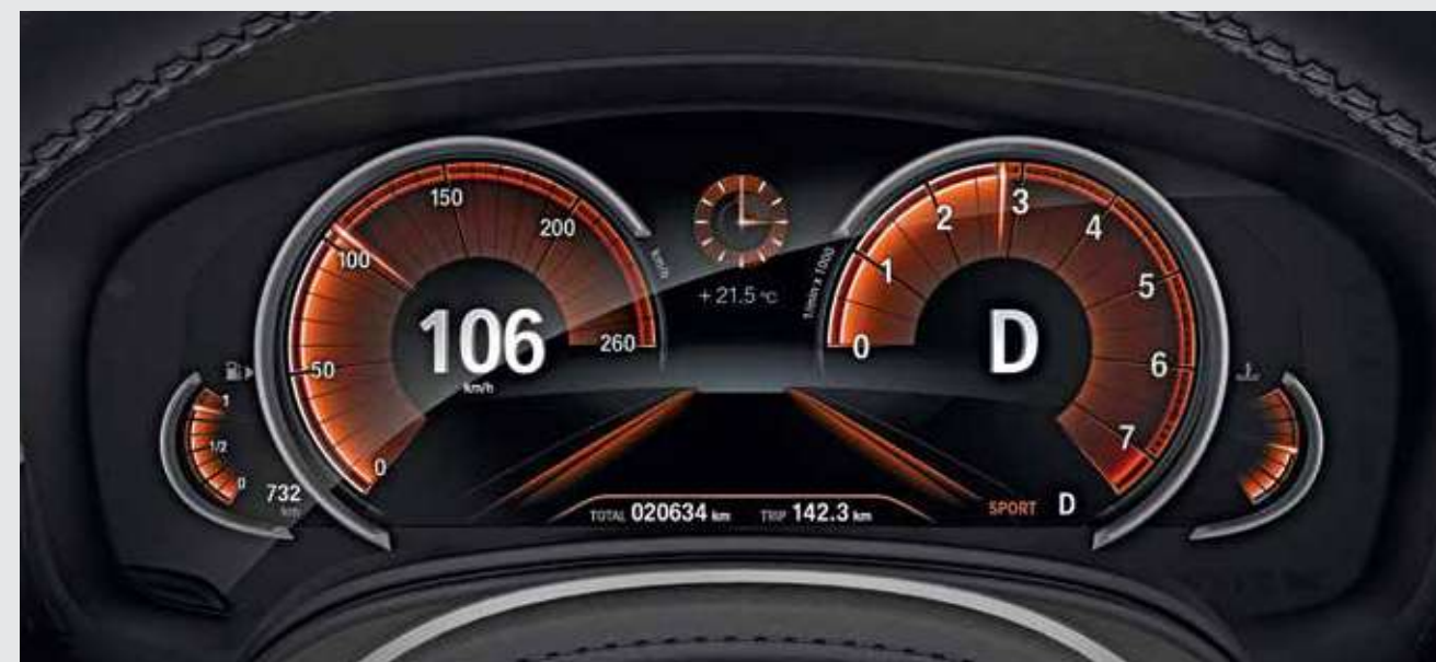
The Multifunction Instrument Display with Black Panel technology and a screen diagonal of 31.2 cm (12.3") provides a highly impressive visualisation of the driving experience. The different modes and their specific displays – each of which have their own colour scheme and graphic style – can be displayed in the instrument cluster.
