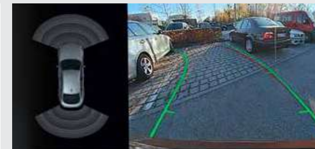
The Rear-View camera enables improved orientation when reversing at speeds below 15 km/h, for example when parking. It shows the area behind the car on the Control Display. Interactive track lines for measuring distance and turning circles assist the driver when manoeuvring, obstacles are marked in colour.
