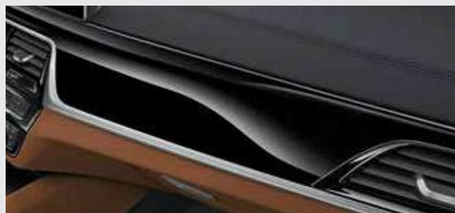
The Instrument panel in Sensatec lends the interior of the vehicle a highly exclusive atmosphere. The artificial leather is applied directly to a semi-rigid foam and features an impressively soft surface.
