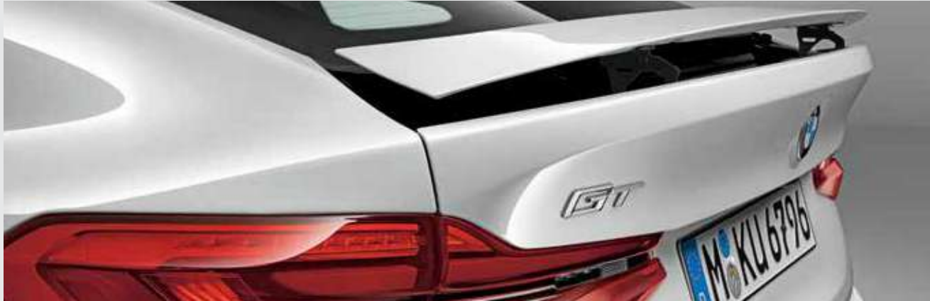
The Active Rear Spoiler automatically extends at a speed of over 110 km/h and retracts once the speed returns to 70 km/h in order to improve stability. It can also be manually activated via a button on the driver's door.
