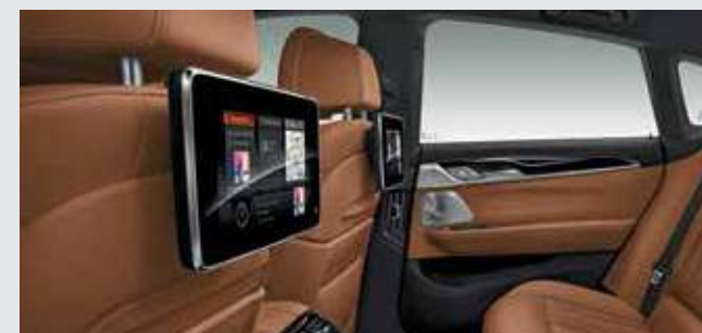
Rear Seat Entertainment Professional includes two separate 10.2" colour screens that can be tilted and a Blue-ray drive. This makes it possible to use the navigation system or the Internet while on the road (with an existing mobile phone contact). Features remote control, USB port and ports for MP3 players, game consoles and headphones (including wireless headphones 3 ).
