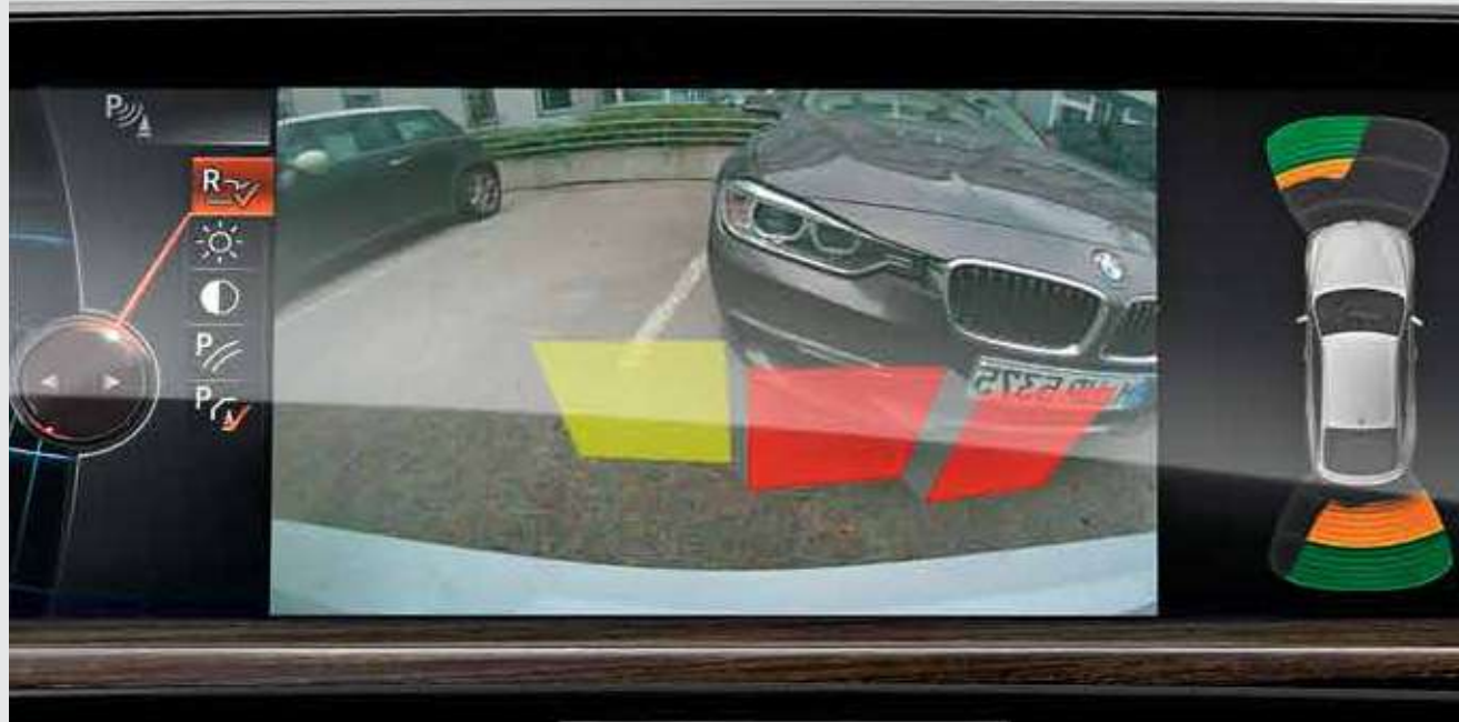
Park Assistant 1 : The park assistant facilitates manoeuvring into parallel and lateral parking spaces. For this purpose, the system measures potential parking spaces while driving by at speeds below approx. 35 km/h even without prior activation.
