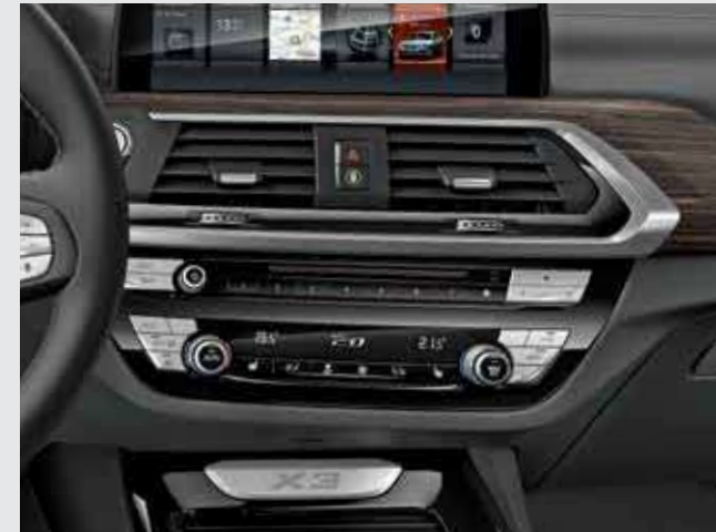
Automatic air conditioning with three-zone control includes Automatic Air Recirculation (AAR) with a micro active carbon filter, as well as fogging and solar sensors.
